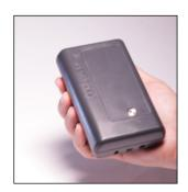
The microAeth® MA200 is a compact, real-time, wearable 5-wavelength UV-IR Black Carbon monitor with a 15 sampling location automatic filter tape advance system which allows for up to 2-3 weeks of continuous measurements.
